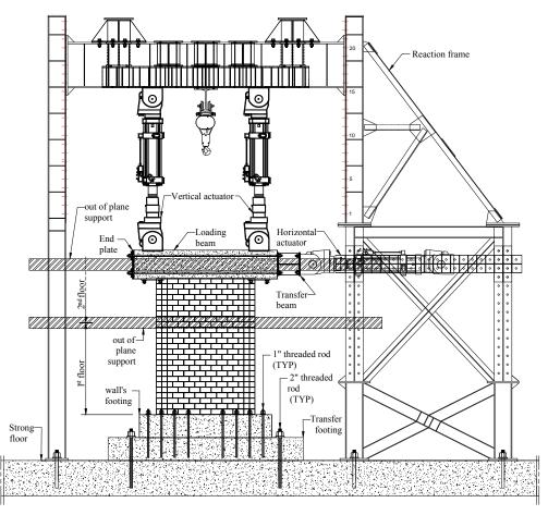
Figure 3. Test set-up
