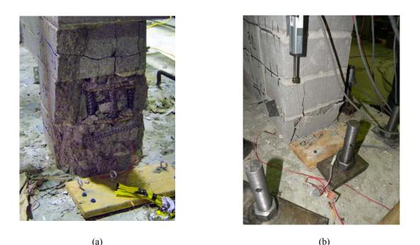
Figure 4. wall failure: (a) bar buckling and grout crushing in wall 4 at  $13\Delta y$ , (b) vertical cracks in the boundary element in wall 6 at  $8\Delta y$ .
